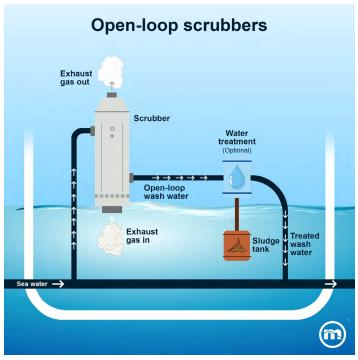
These systems utilise seawater with a natural alkalinity to neutralise sulphur oxides in the exhaust gases. Once treated, the wash water is released back into the sea as long as it complies with the discharge regulations set by MARPOL.
