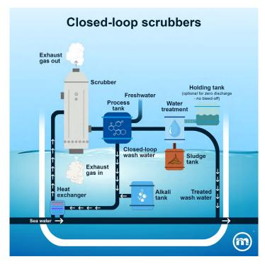
These systems use fresh water and chemicals like caustic soda to increase alkalinity. The water is recirculated within the system, with periodic purging of a small portion. Accumulated sludge is stored onboard for proper disposal at port facilities.
